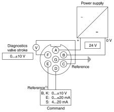
1) Do not connect with supply voltage zero.
